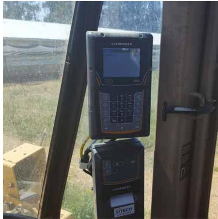
Trimble LOADRITE L2180 loader scale connected to InsightHQ reporting and printer installed in-cab
